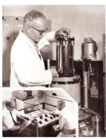
The calculations involved plotting these on large graphs (4 or 5 feet by 2 feet) and measuring areas with a planimeter. This was for special accurate measurements with a gold plated bomb. For routine cordite samples an automated bridge was used".
