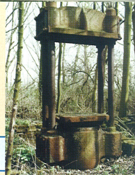
Left: Hydraulic pump mechanism for press driven by water wheel, 1940
