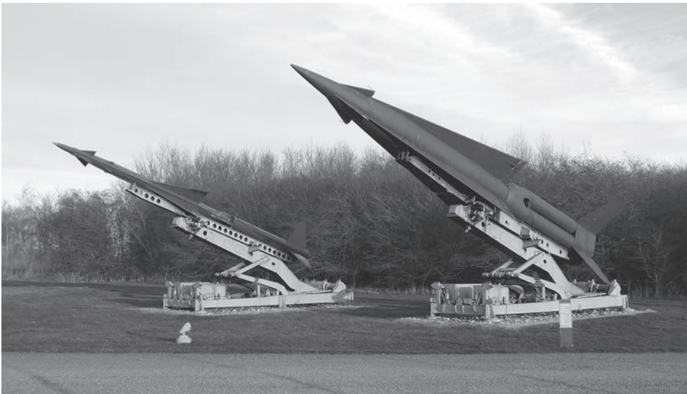
Fig. 35 Stevns Fort, Denmark, the Cold War museum displays a number of surface to air missiles, to the left a Nike Ajax and to the right a Nike Hercules. From 1960 until the 1980s both types defended Copenhagen. (© Wayne D Cocroft)
