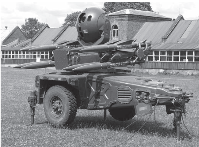
Fig. 13 Rapier missile and tracking unit, a modern fully mobile surface to air missile system requires little if any fixed infrastructure. (© Wayne D Cocroft)
