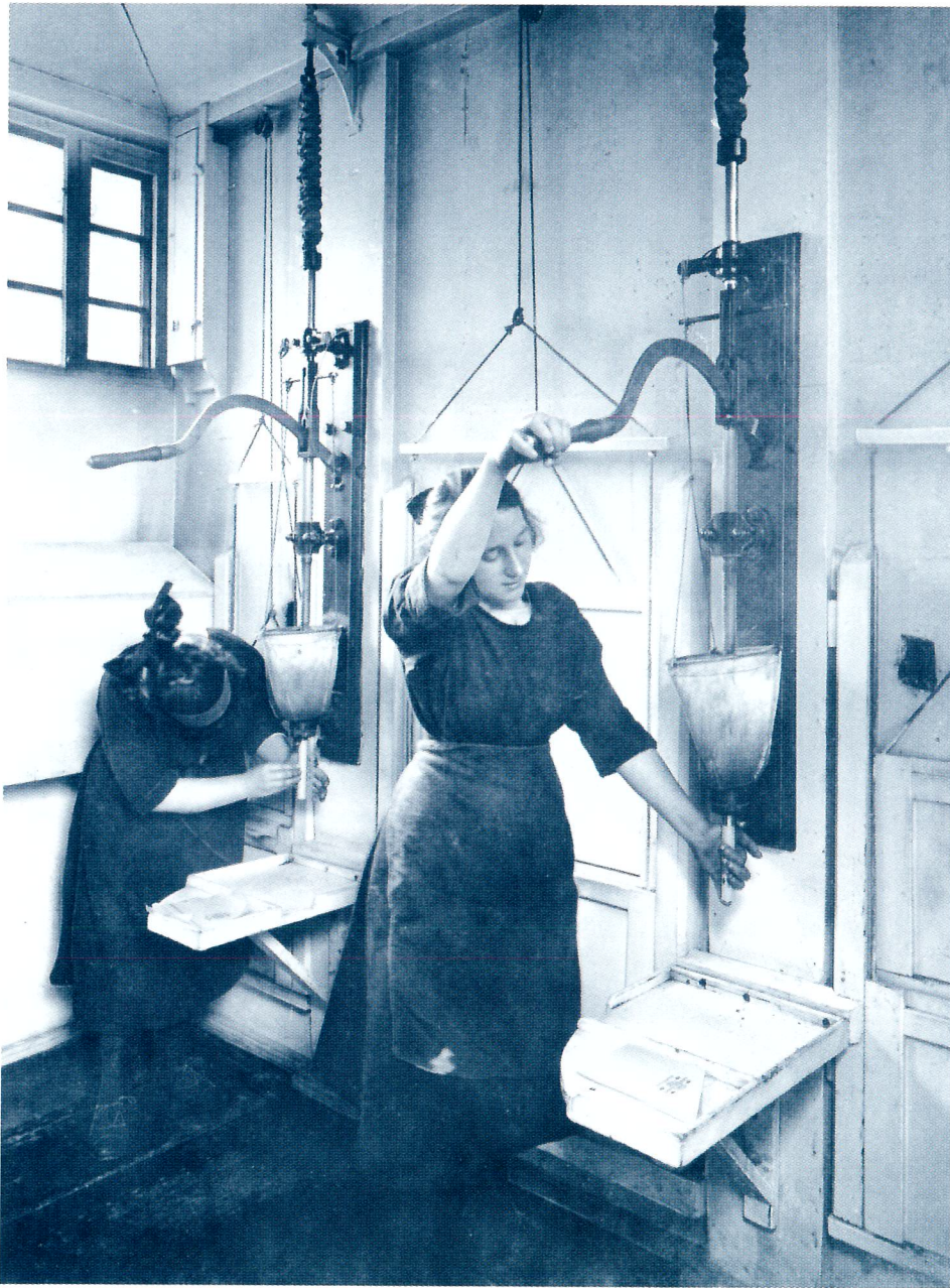
Plate 16: Detailed view inside a Dynamite Cartridgeing Hut, circa 1925, showing an original Dynamite cartridgeing machine in use (ICI Explosives, C65509)
