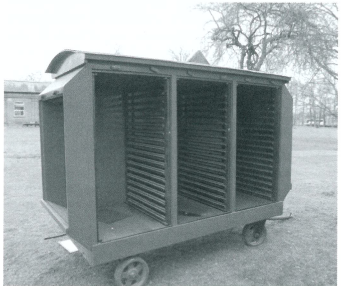
Fig. 7 Rebuilt Cordite drying wagon.
