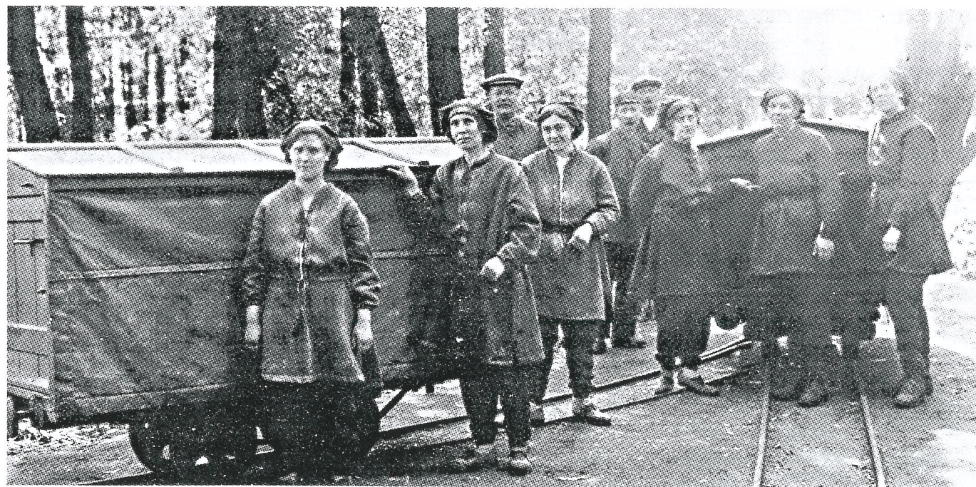
Hand-propelled wagons with peaked roofs, probably photographed during World War 1. These smaller wagons were used within the process areas. (RARDE)
