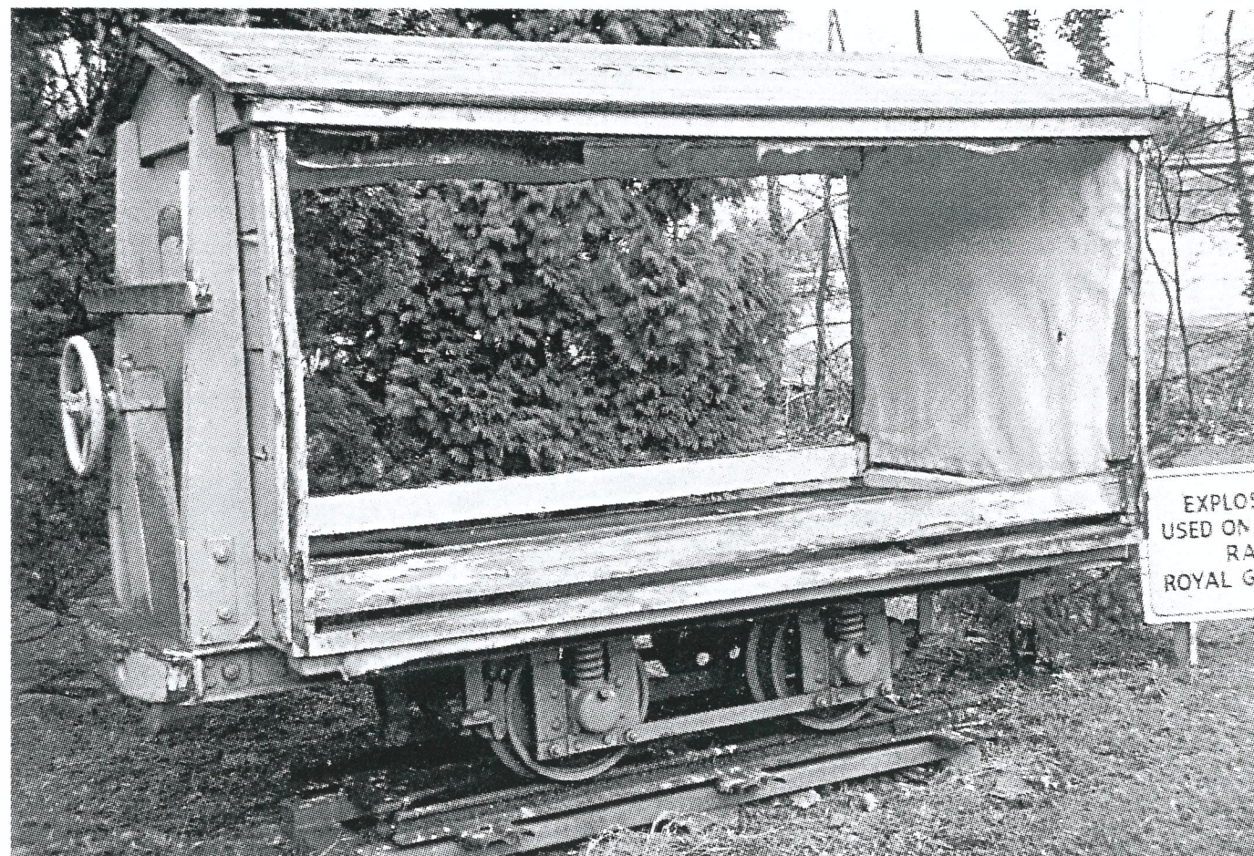
The most substantial relic of the Royal Gunpowder Factory railway is this Hudson-built cordite paste wagon, preserved on the RARDE North Site. (J.M.Jenkins)
