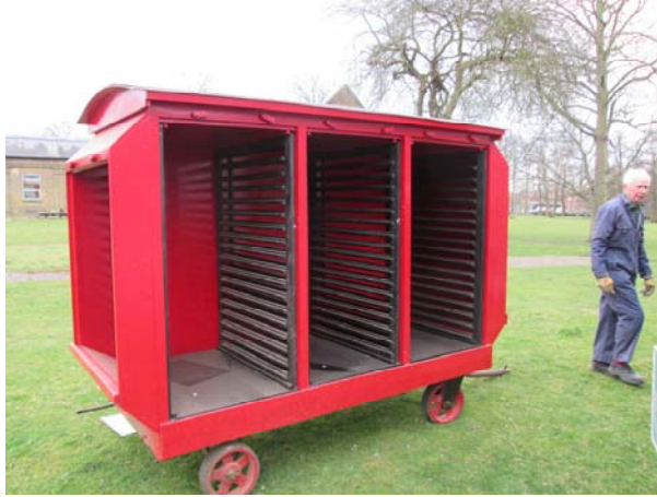
Fig 6 Rebuilt Cordite drying wagon
