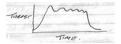
The oscillations are a function of the rig which 'rings' like a bell. Modern computer programmes could subtract this ringing waveform from the raw data to give the 'true' thrust/time curve
