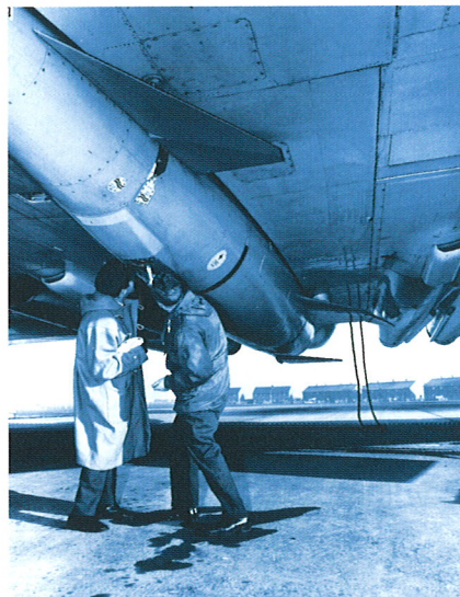
Figure 2.15 Blue Steel standoff bomb secured to a Vulcan aircraft, c. 1965. Each Vulcan carried a single Blue Steel standoff bomb in a modified bomb bay. The bomb's ventral fin was folded during takeoff and deployed when the bomb was released from the aircraft. (Crown copyright)
