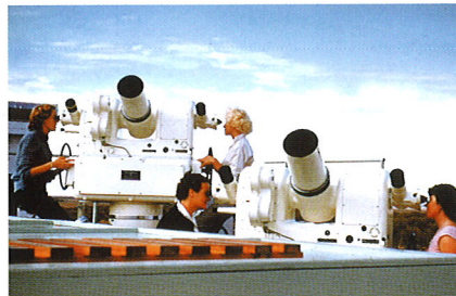
Figures 3.7 and 3.8 Contraves kinetheodolites, c. 1965. Kinetheodolites are used to track the launches of missiles and space vehicles. The ones shown here were used on the Blue Streak programme. They provided a cine-film record of the vehicle synchronised to its angle and direction of flight. (Commonwealth of Australia)
