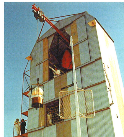
Figure 4.4 Black Arrow R1 launch. The nose-cone fairings were painted orange to increase their visibility. The line markings on the first stage enabled the tracking cameras to record the vehicle's degree of roll. (Commonwealth of Australia)
