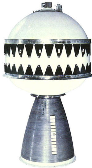
Figure 3.4 A Waxwing rocket motor, c. 1966. The Waxwing's shape was the first of its kind in British rocketry. Its near-spherical form enabled the smallest amount of steel casing to be used for a given quantity of solid propellant contained within. The nozzle was also gently arced in a near 'Rau' design, not previously used in Britain, to improve its performance. (BAE SYSTEMS plc)
