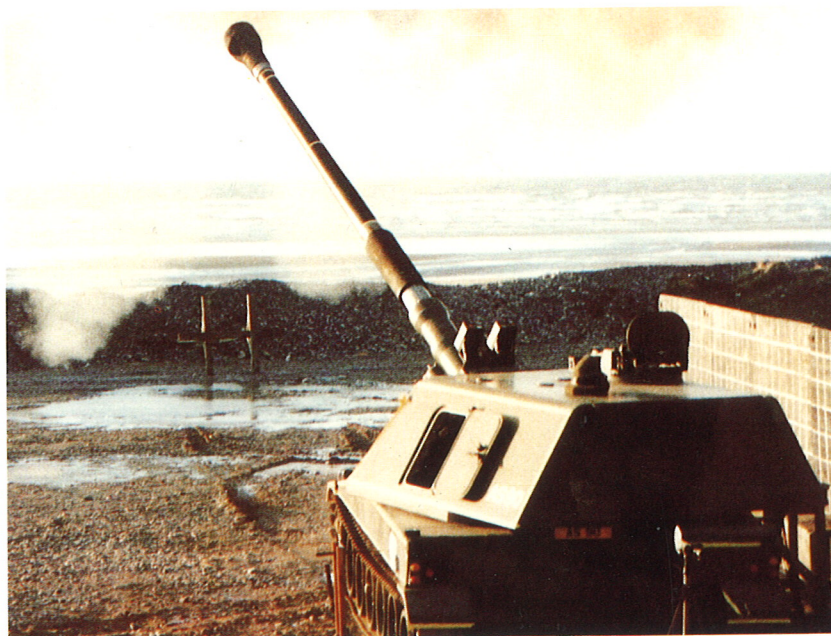
Self Propelled Artillery. AS90, which is VSELs front running contender for the British Army will mount the Royal Ordnance 39 Calibre 155mm gun system.
