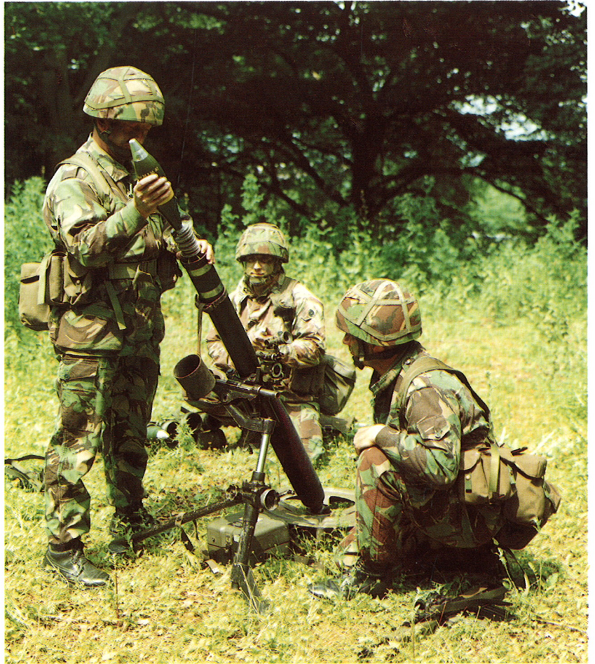
The 81mm Mortar provides lightweight manportable firepower for the infantry out to a range of over 5600m.
