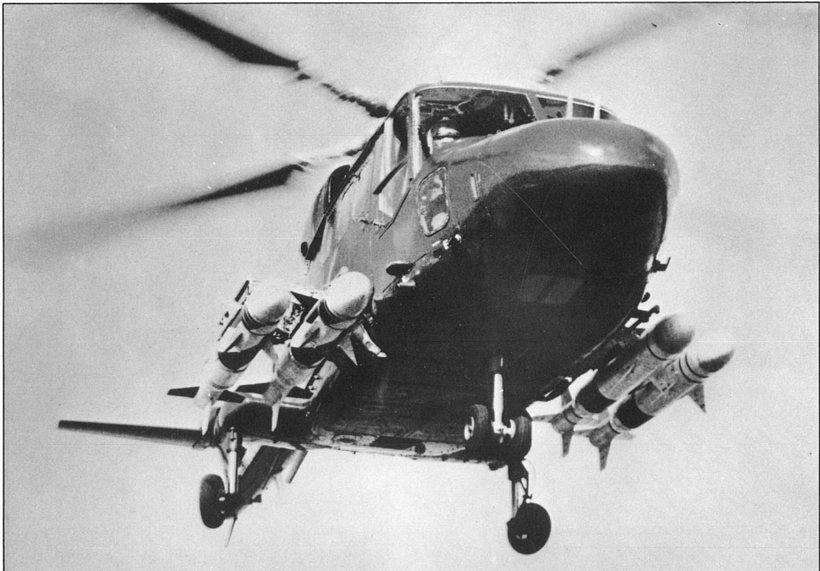
BAe Sea Skua anti-ship missiles. Boost and sustain rocket motors by the Explosives Division.
