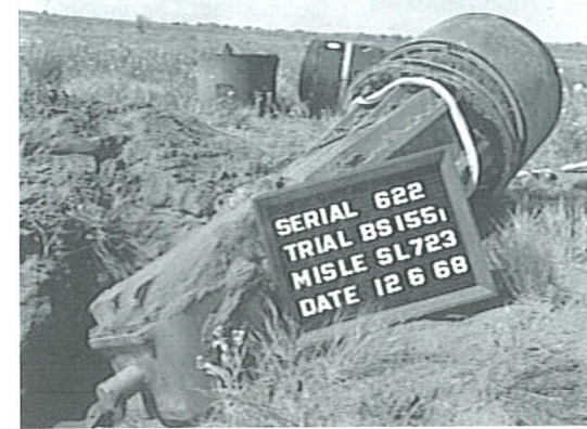
A recovered instrument section of a Skylark rocket from the Australian desert.
