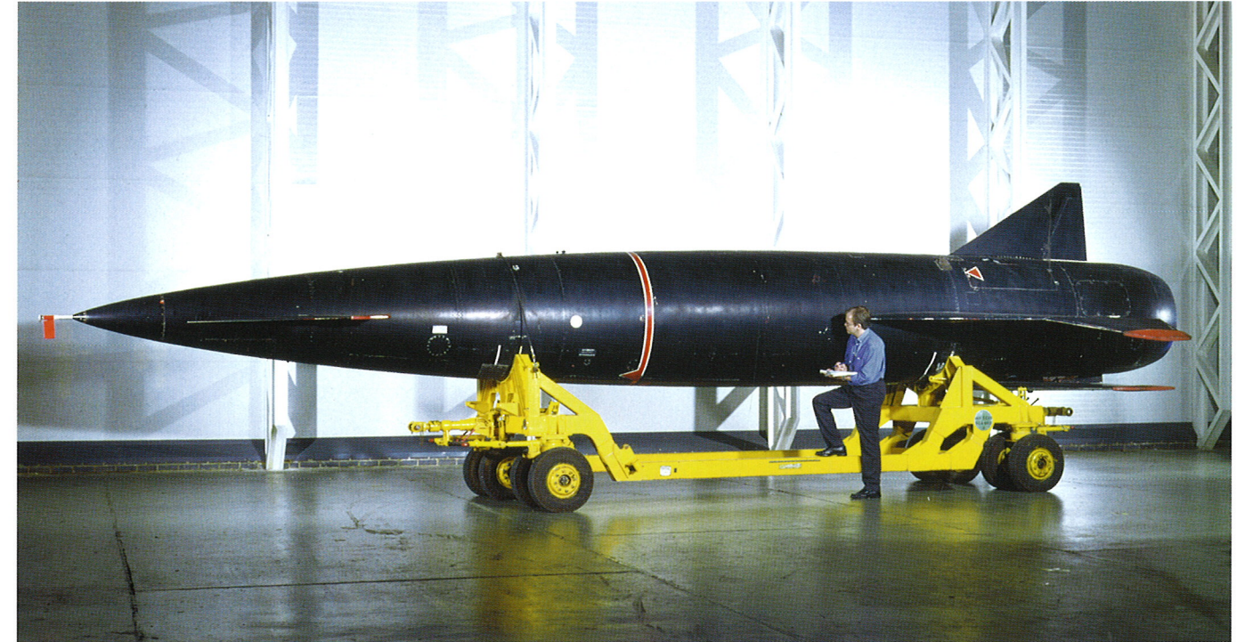
Figure 2.14 Blue Steel standoff bomb, c. 1958. The Science Museum's Blue Steel rocket was a test vehicle and is fitted with a Double Spectre engine (see Figure 2.12). It would have been air-launched from a Vulcan aircraft and flown over a restricted range to test its performance (Inventory No. 1987-0752). (Science & Society Picture Library)
