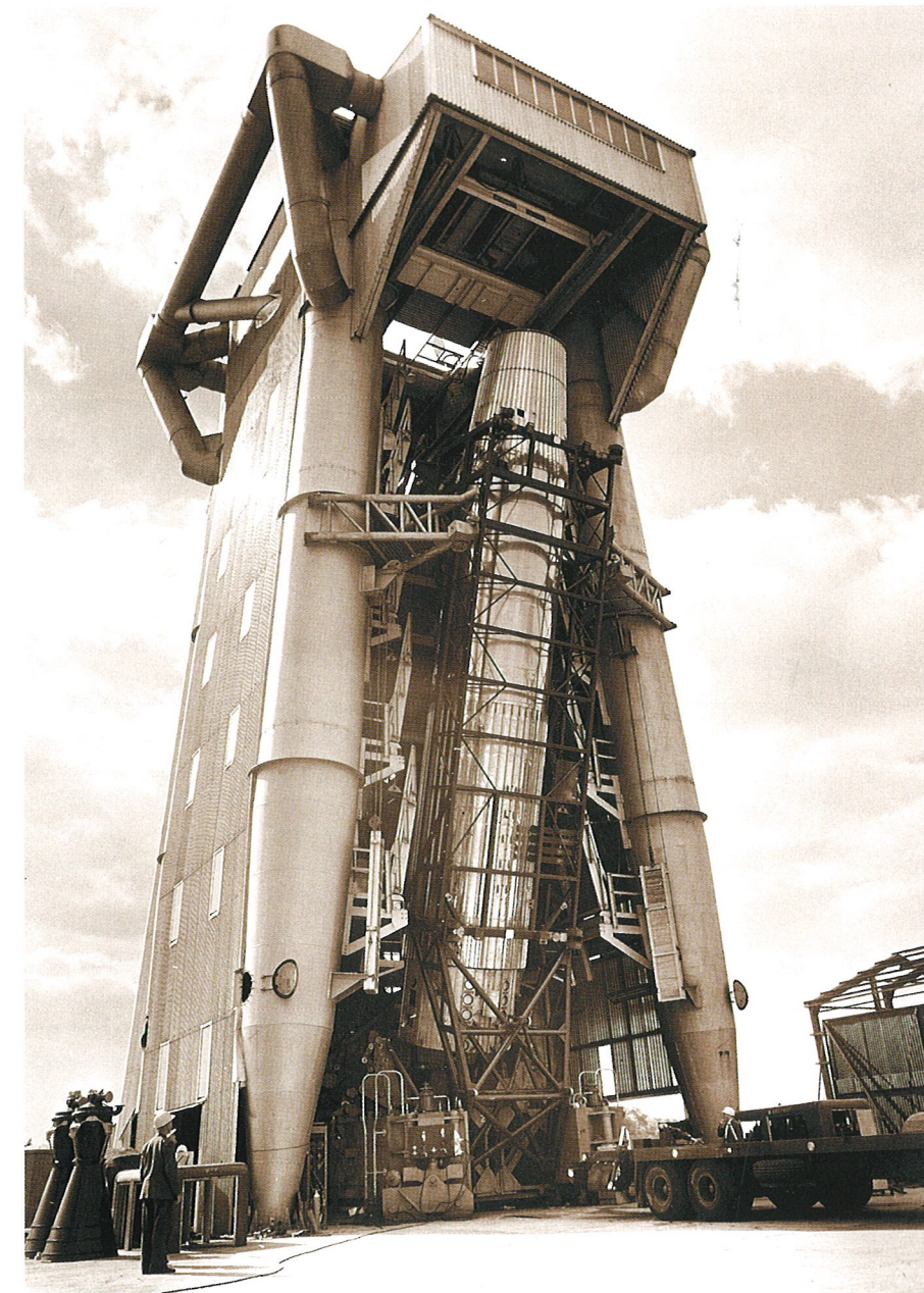
Figure 1.4 An early Blue Streak development vehicle being raised into position for testing at De Havilland Propellers' Hatfield site in Hertfordshire, England, c. 1959. Blue Streak was based on the United States' Atlas missile, and was fitted with RZ-12 engines that burned kerosene in liquid oxygen. Transatlantic agreements allowed British companies, helped by the Royal Aircraft Establishment, to acquire information from their United States equivalents. This enabled these companies to develop the Blue Streak vehicle. De Havilland Propellers Ltd liaised with Convair on the vehicle itself, while Rolls-Royce exchanged information with the Rocketdyne division of North America Aviation. (Astrium)
