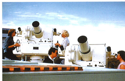
Figures 3.7 and 3.8 Contraves kinetheodolites, c. 1965. Kinetheodolites are used to track the launches of missiles and space vehicles. The ones shown here were used on the Blue Streak programme. They provided a cine-film record of the vehicle synchronised to its angle and direction of flight. (Commonwealth of Australia)
