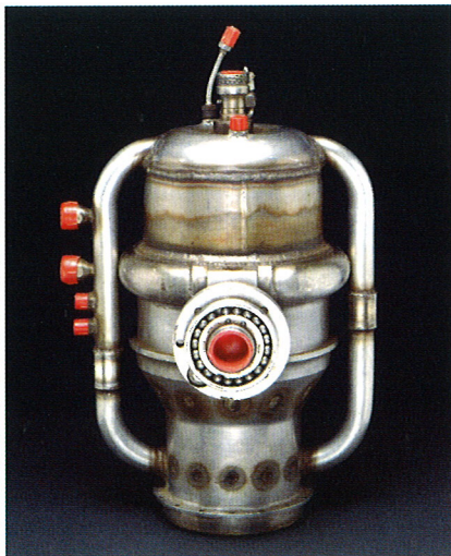
Figure 5.5 A more likely proposal for a Black Arrow upgrade would have relied on more powerful Gamma engines. The photograph shows a Larch (large rocket chamber) (c. 1968), a Gamma upgrade that could deliver 7500 lb (3400 kg) of thrust (Inventory No. 1983-836). (Science & Society Picture Library)
