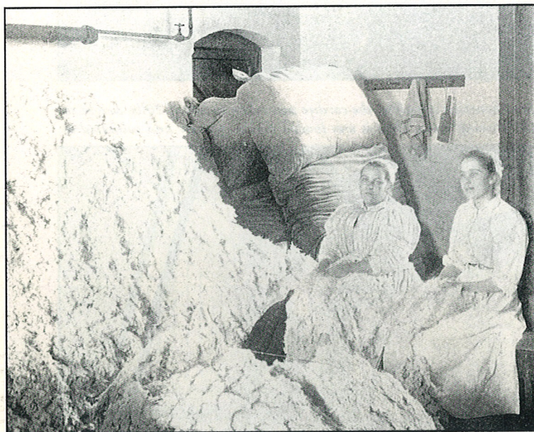
Fine cotton waste from the textile factories of the North was carefully hand picked and shredded to remove foreign bodies before being placed in a vast oven. Here it was revolved on racks which passed constantly up and down through the drying area for twenty minutes in a temperature of 180 degrees. On leaving the oven, packs weighing just over 11b were sent in bins to the nitrating plant where they were allowed to fall into baths of mixed acid.
