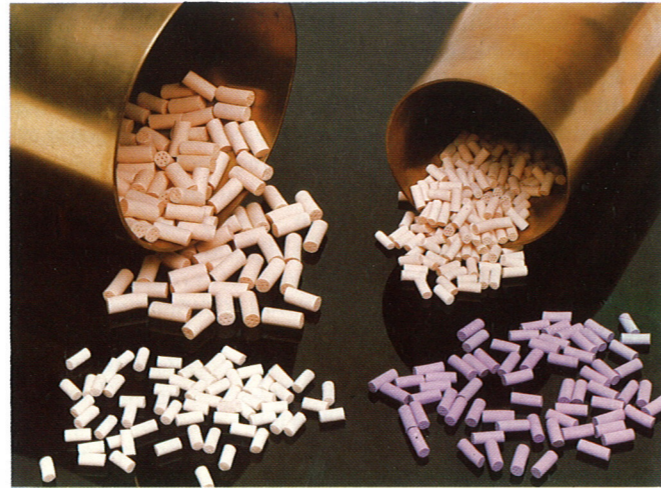
Slotted tubular granular propellant
