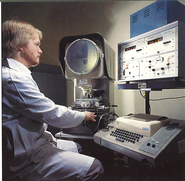
The analysis of high speed detonation photographs to assess the performance and characteristics of explosives.
