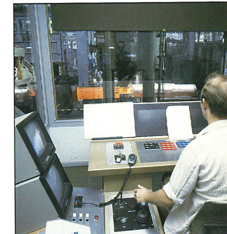
The new computer controlled gun forge at Nottingham has significantly improved the Division's capability to manufacture high quality barrels from 76mm to 155mm.
