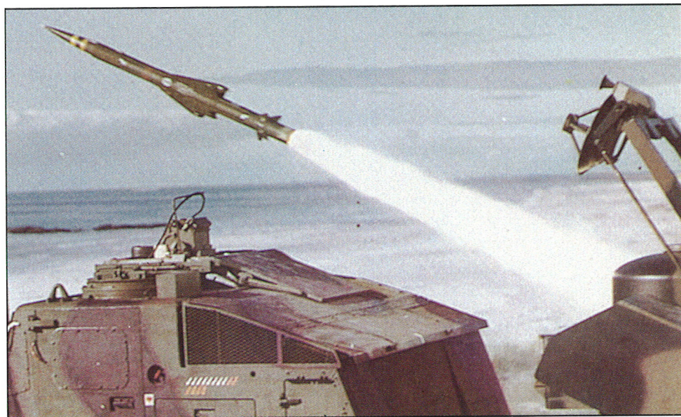
Launching the tracked Rapiers missile, powered by a Troy dual thrust motor, designed and manufactured by the Division. Motors are designed to operate in variable environmental conditions and have long service life, high reliability, low smoke emission and the option of thrust vector control.
