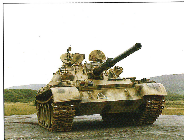
Royal Ordnance has designed a family of regunning kits to improve the effectiveness of the Russian- and Chinese-built T series battle tanks. At present, work is being carried out on the T55 tanks of the Arab Republic of Egypt.
