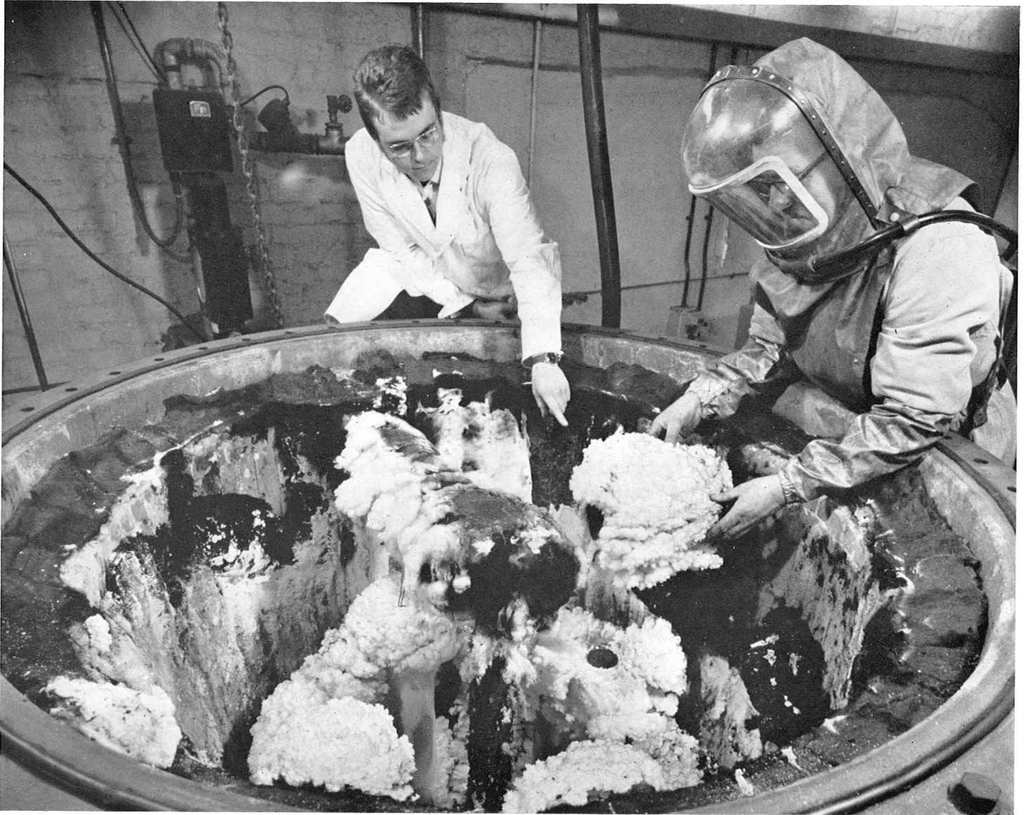
Removing silicon nitride whiskers from one of the experimental high temperature reactors at ERDE
