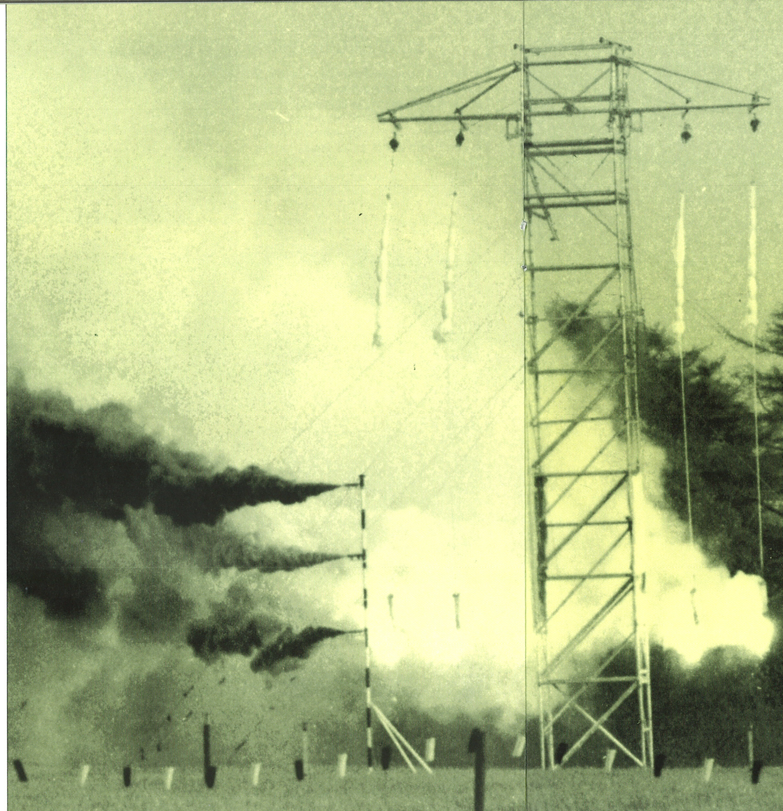
A solid propellant rocket firing showing secondary combustion
