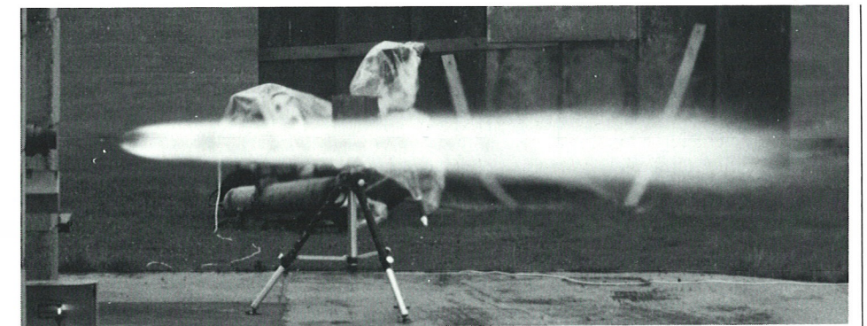
A solid propellant rocket firing showing secondary combustion
