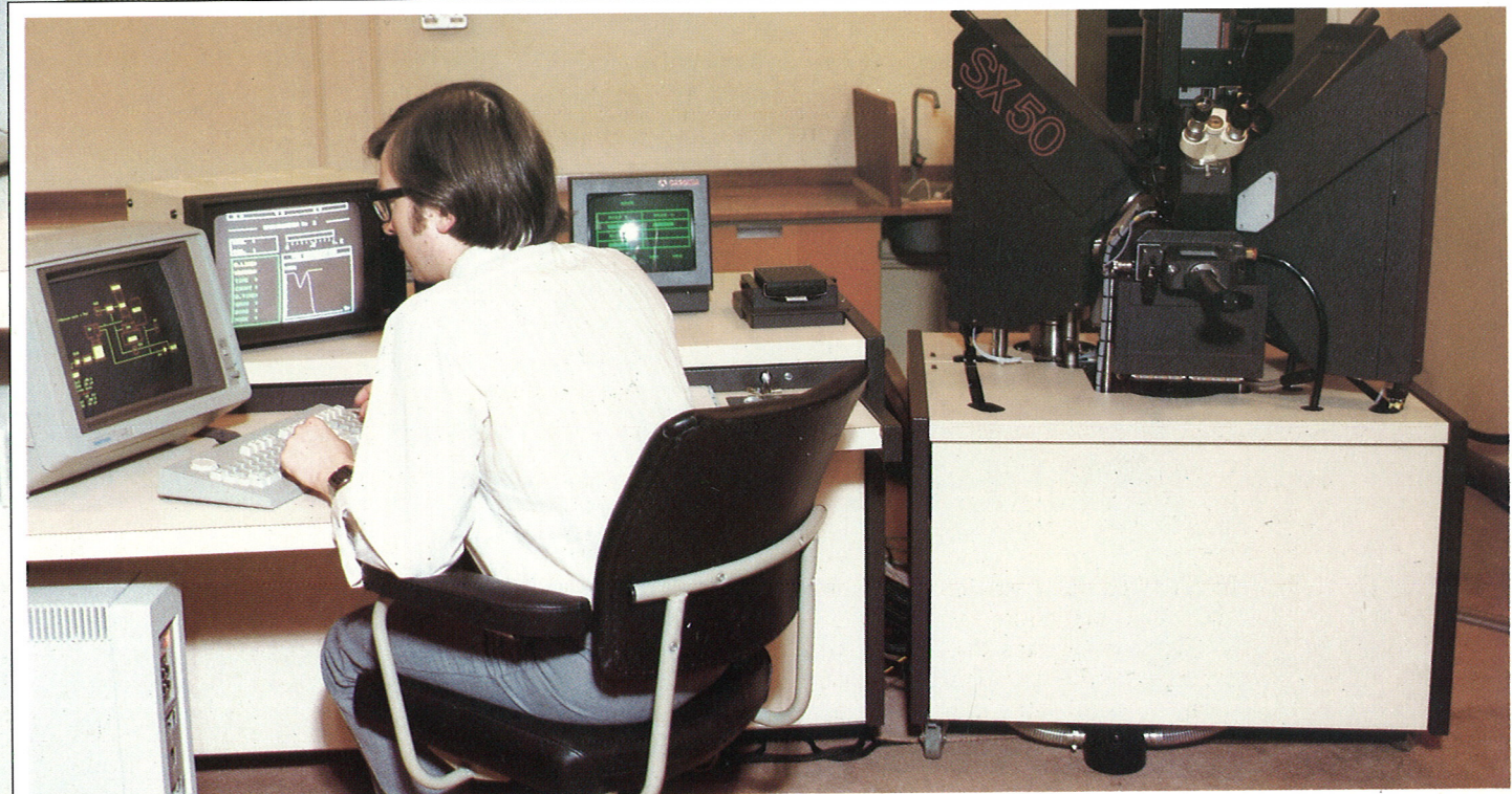
Collation of output from Electron Probe Microanalyser provides analysis of surface areas down to 1/1000 mm. diameter.
