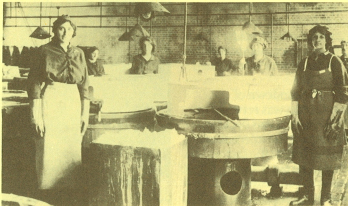
Guncotton nitration by displacement process
