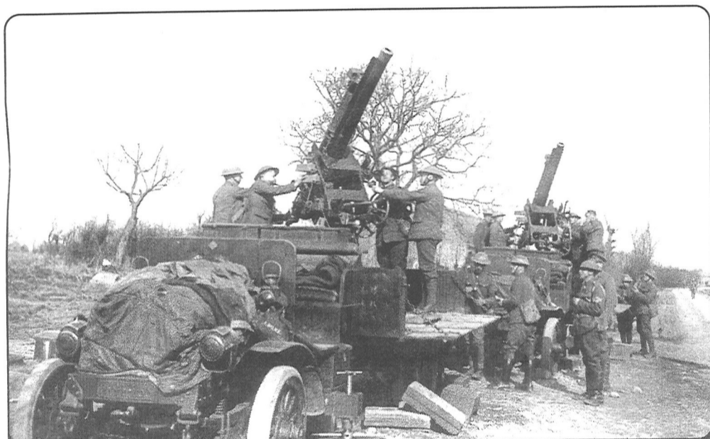
The 13-pdr 9cwt gun was widely employed in a mobile role. Here it is seen mounted on Peerless lorries in March 1918 (IWM Q.8559)
