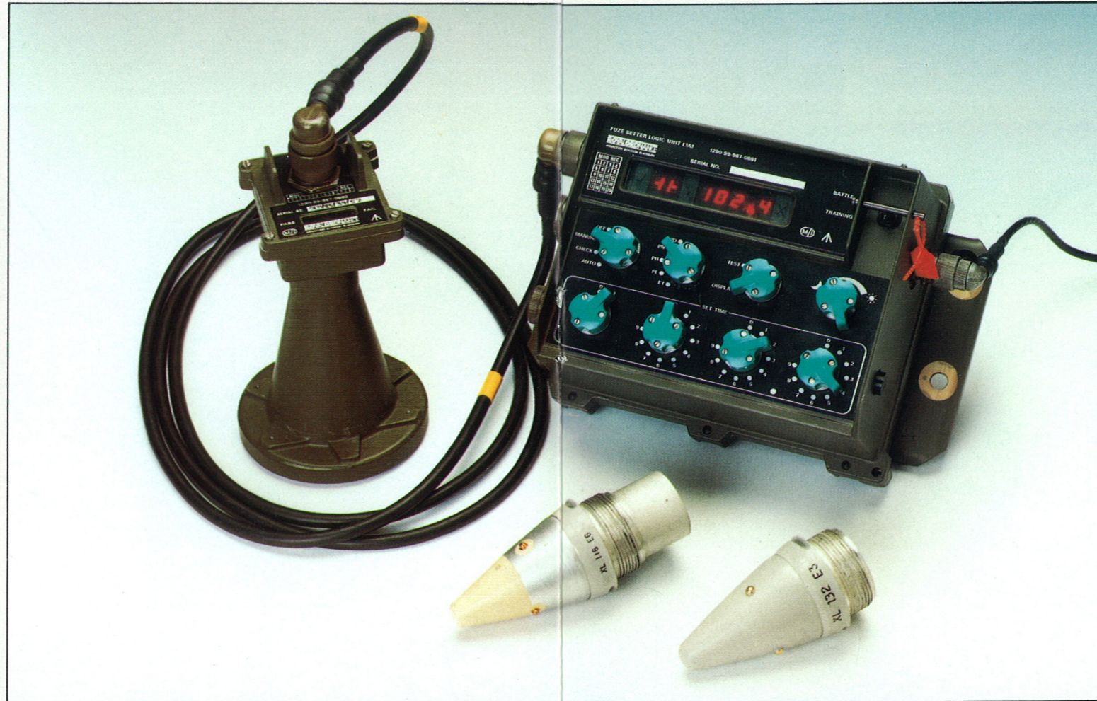
Fuze-setter for Multi-Role and Electronic Timed Fuzes.
