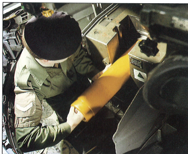
Loading of propelling charge for 120 mm APFSDS ammunition, developed by Royal Ordnance Explosives Division.
