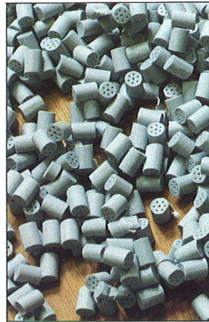
Multi-tubular granular propellant.
