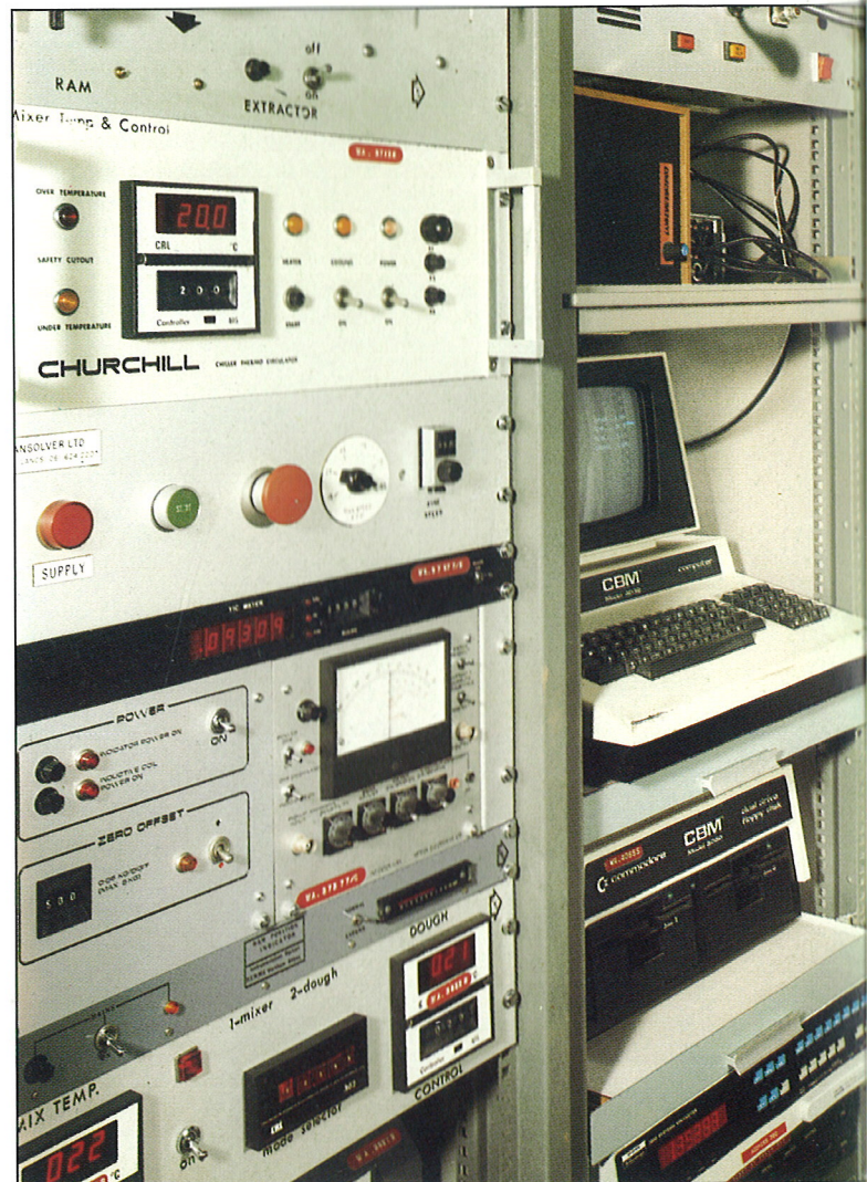
Control console for research into new methods of instrumented propellant mixing.
