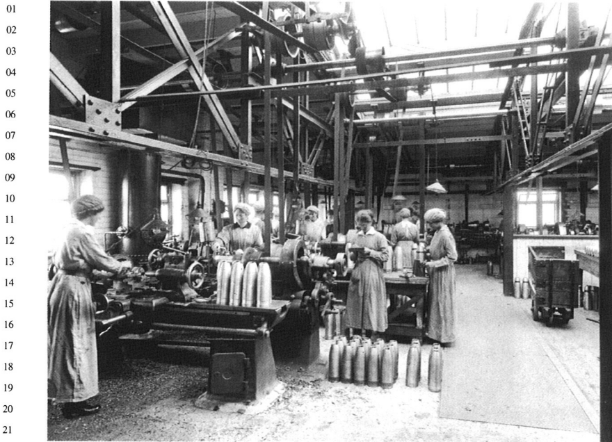
23 Figure 4. In this view of the top floor of the Cunard's Shellworks, Liverpool the women are working 24 on 4.5-inch shells. In the foreground the operator is cutting a groove at the base of the shell ready to 25 accept the copper driving band. On the adjacent lathe the operator is using a gauge to test the depth 26 of the cut and on the centre bench the dimensions of the shell are being checked with another gauge (BL24001-21). © Crown copyright.NMR
