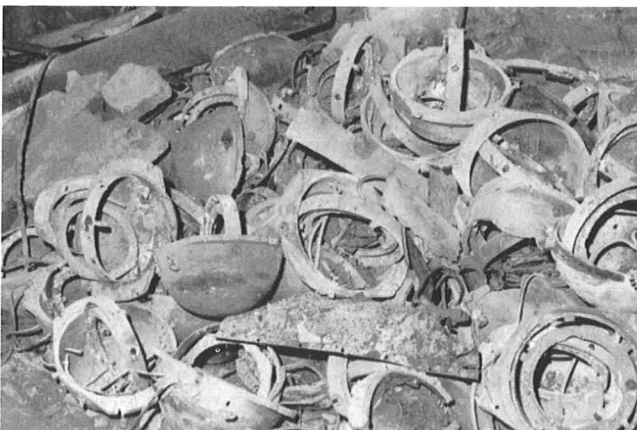
Left: A heap of spherical holders for the V1 magnetic gyro compass and (right) a V1 fuel tank.
