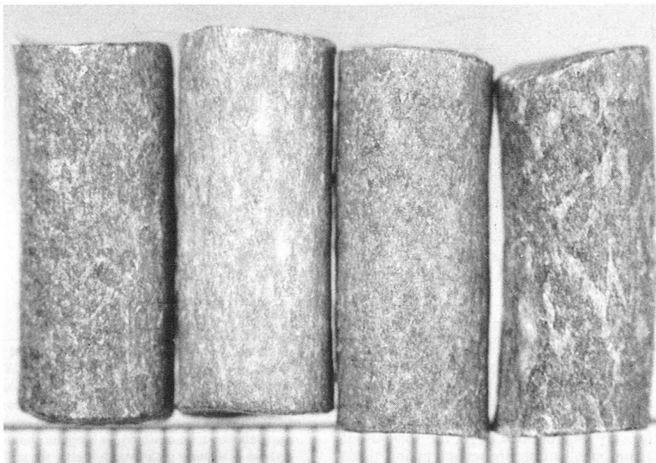
Elevation and end view of a few large grains of propellant suited for a medium calibre field gun. The distortion caused by the loss of solvent on drying is clearly visible in such large grains, as is the lack of a surface coating — in cannon powders any moderators etc are normally incorporated in the mix during manufacture. The scale divisions are in millimetres.
