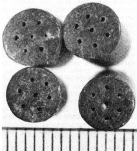
Elevation and end view of a few large grains of propellant suited for a medium calibre field gun. The distortion caused by the loss of solvent on drying is clearly visible in such large grains, as is the lack of a surface coating — in cannon powders any moderators etc are normally incorporated in the mix during manufacture. The scale divisions are in millimetres.
