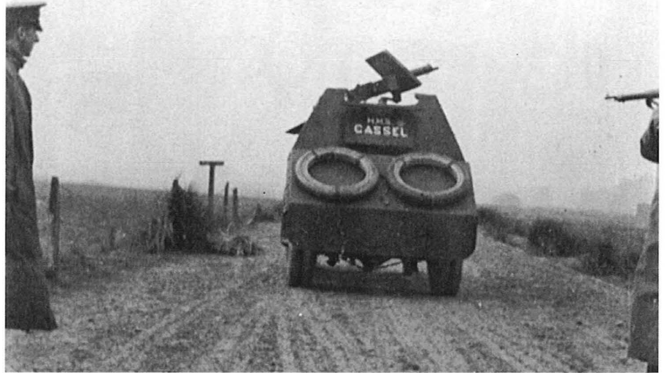
One of the improved, armoured Talbots, which Samson named after an earlier action, is subjected to a rough but effective test of its armour. Notice the greater flexibility of the new Maxim mounting.
