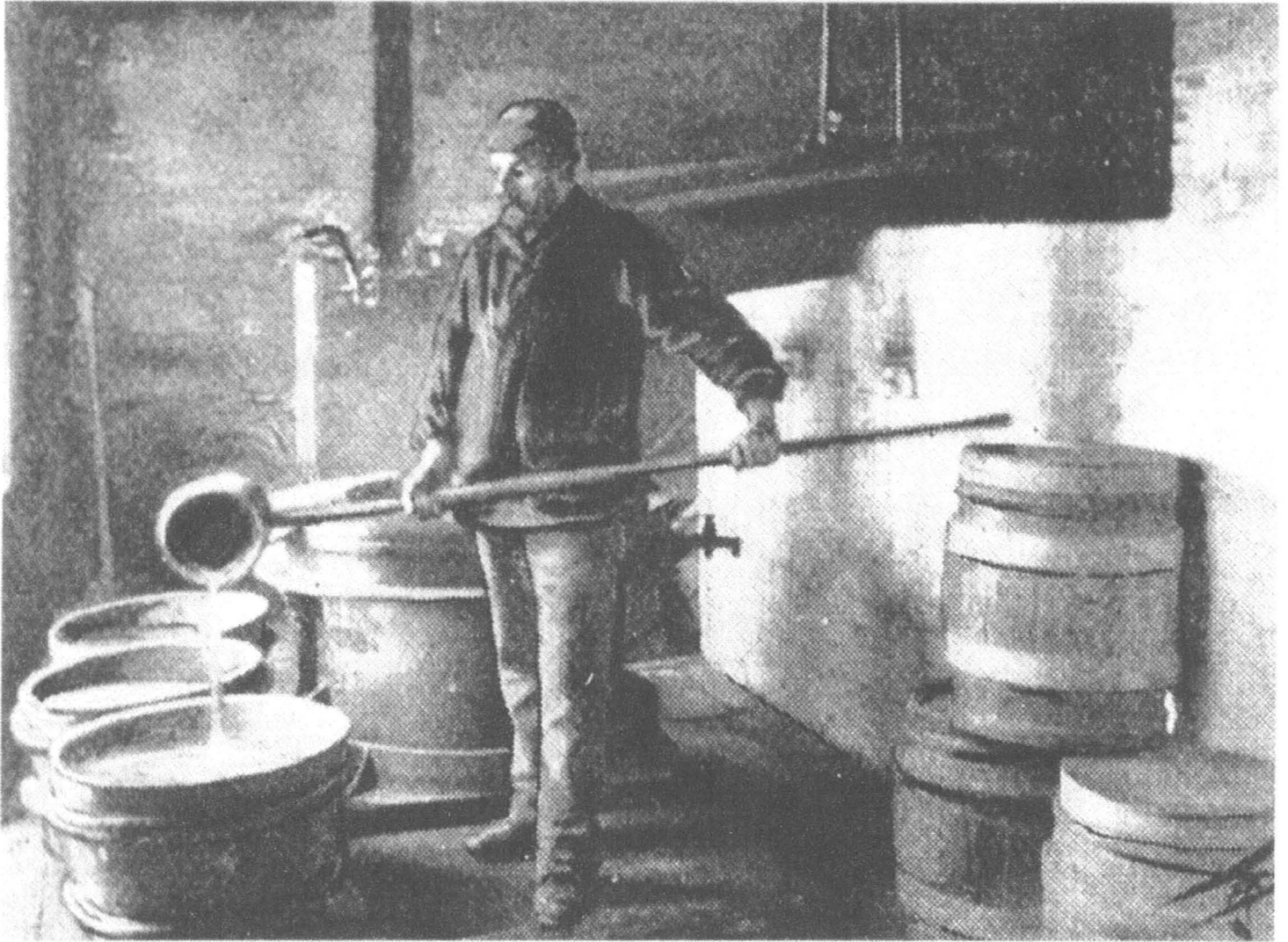
Ladling liquid sulphur into wooden tubs from the receiving pot of the distilling plant at Waltham Abbey, 1895.
