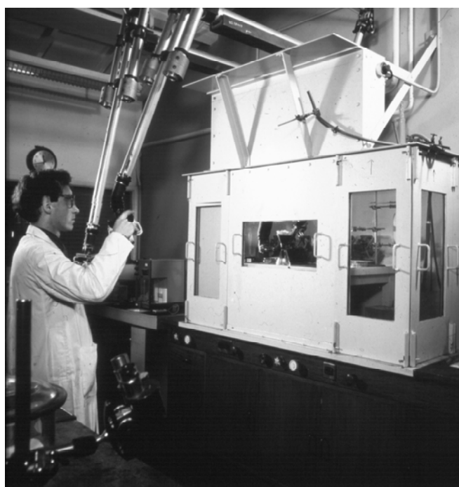
Fig. 8. Explosives cabinet with remote handling.
