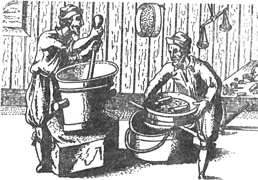
Mediaeval powder-making: (left) pestle and mortar being used to "incorporate" the sulphur, saltpetre and charcoal as closely as possible; (right) using a sieve to "corn" the powder into uniform-sized grains. (Courtesy of I.C.I.)
