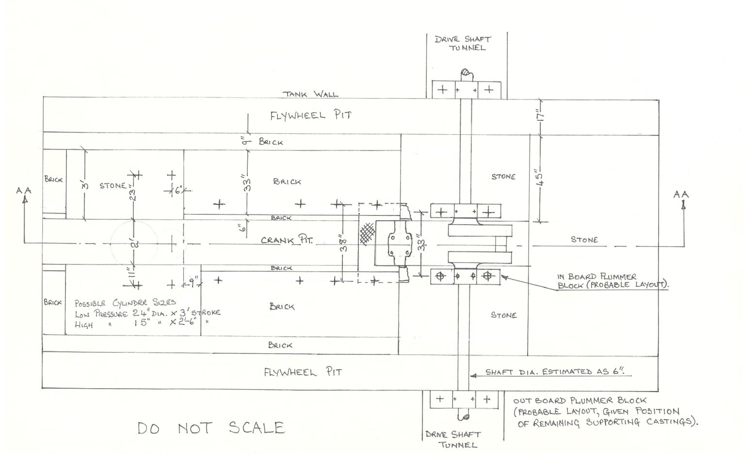
BEAM ENGINE GENERAL LAYOUT. SCALE 1/2"=1 FT. DRAWN BY J: WILSON 19TH JULY 2001. DRAWING 3 OF 3.
