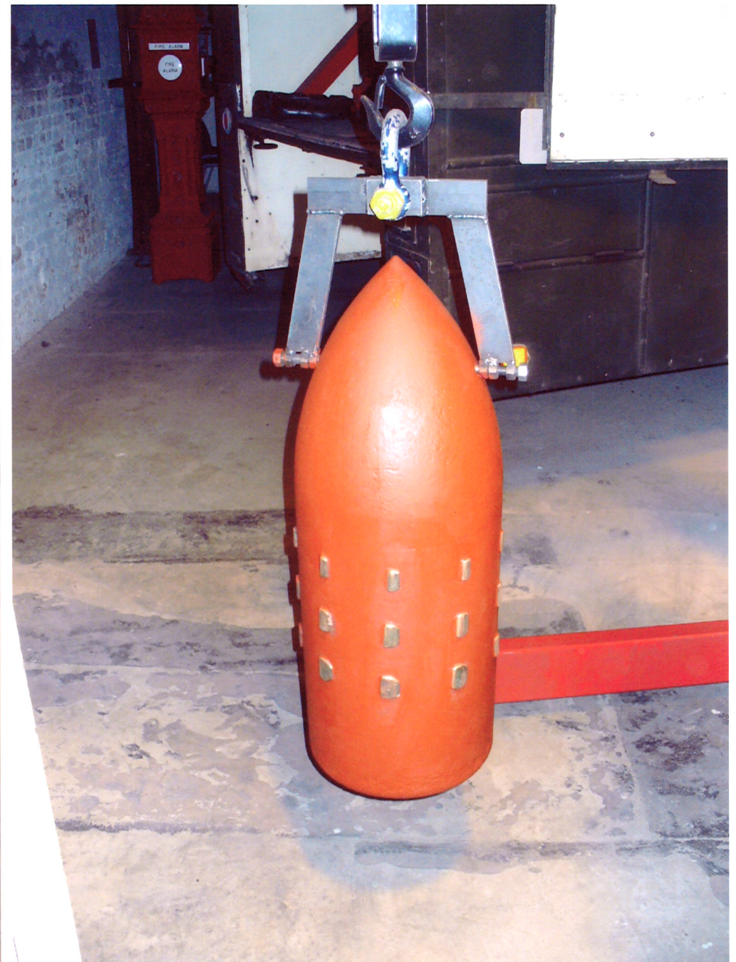
Two views of 12" shells after cleaning and first coat of red oxide. 7th. January 2006
