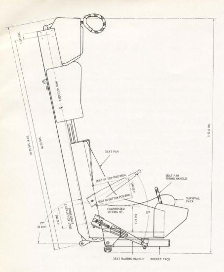
of the aircraft before the ejection seat operates, a half second time delay mechanism is installed in the breech of the ejection gun. When the sear is withdrawn from the time delay mechanism the initial downward movement of the firing pin is controlled by an escapement mechanism until a delay of a half second has elapsed when the firing pin is free to descend, under spring pressure, to strike the percussion cap of the primary cartridge and thus initiate
