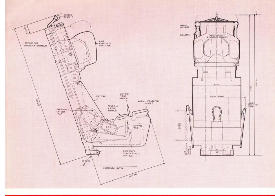
At present under development for the West German Air Force, the VAK 191 V/STOL tactical reconnaissance fighter is to be equipped with the Martin-Baker Mk. 9 ejection seat. The speed range of the aircraft is such that although escape must be possible under zero altitude/zero speed conditions the ejection seat must also be capable of bringing about a safe ejection at speeds in excess of Mach 1.
