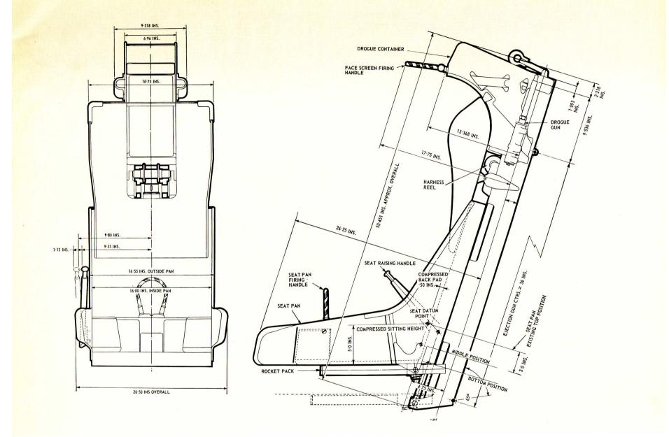
The Martin-Baker Mk V6 ejection seat has been designed for the Short SCI, VTOL experimental aircraft. Owing to the restricted amount of space available in the cockpit the envelope dimensions of the seat have been kept as small as possible. This has in no way affected the function of the seat which incorporates many of the well-proven Martin-Baker ejection seat components.
