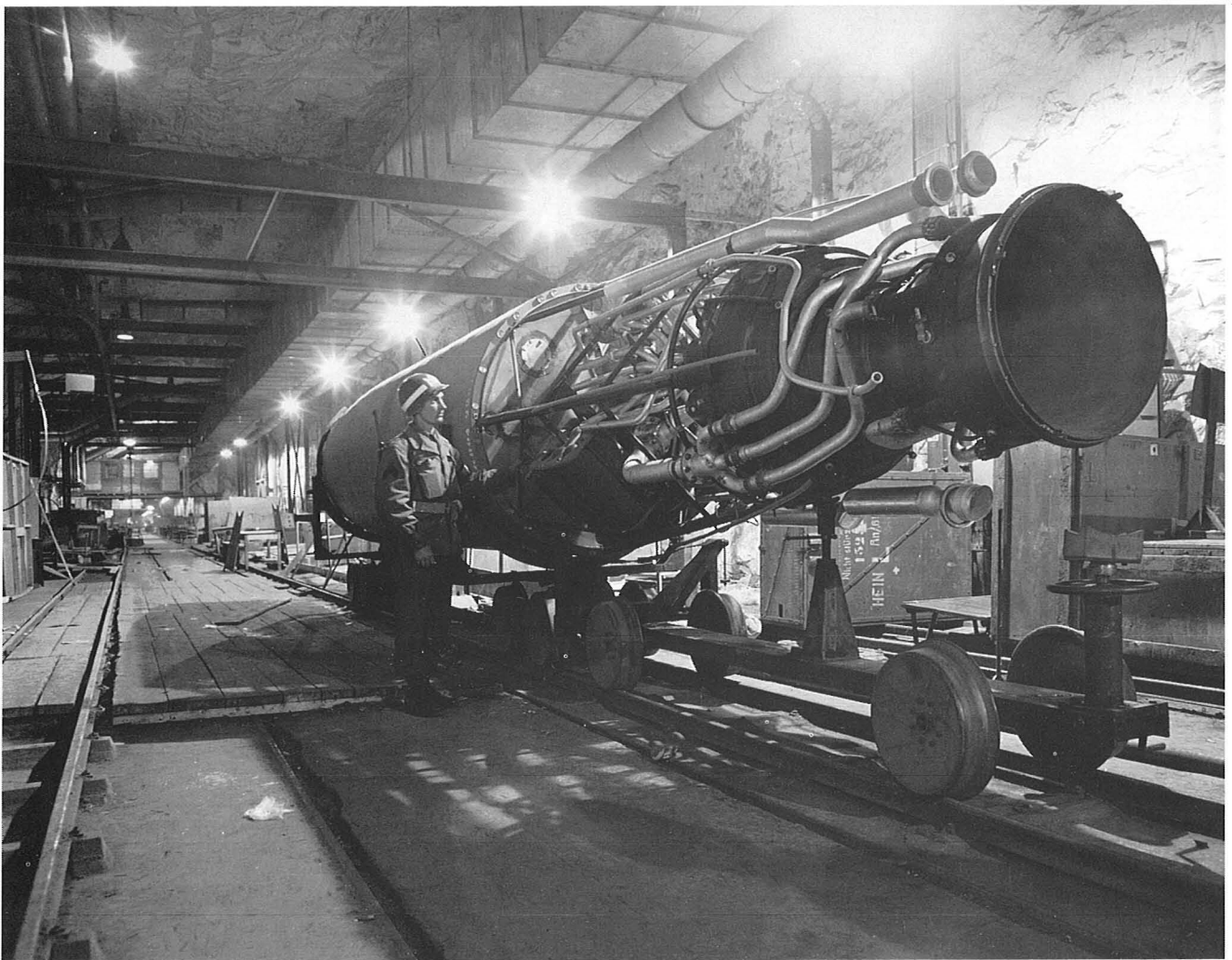
By the time the assembly line in Tunnel B reached this point, the rocket on the trolley was nearing completion. This picture, taken by the Americans after they captured the factory in April 1945, shows one that is complete except for its tail unit. Note the planking on the floor covering a stretch of the standard-gauge rail track. (IWM)
