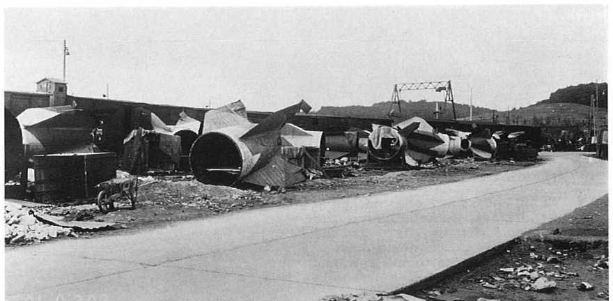
Right: Outside the camp, the Allies found large quantities of V1 and V2 parts, stored in the open for lack of space inside the mountain. These V2 tail units are along the road just before the entrance to Tunnel A (the turn-off can be seen in the distance on the right). The box-car train in the background stands on one of Tunnel A's rail tracks. (BA) Below left: The curve of the camp road helps to pinpoint the spot.
