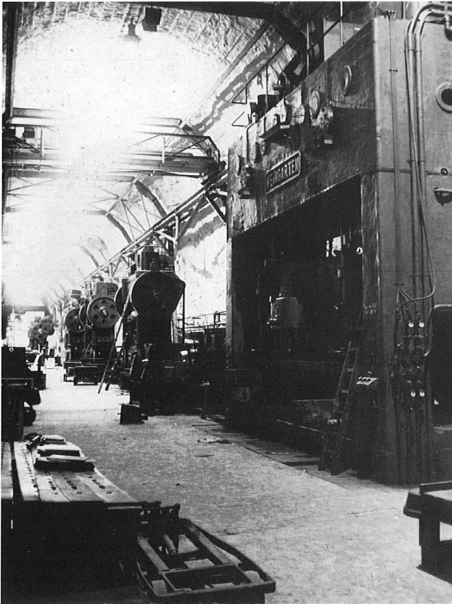
Metal-press workshops were in both Gallery 32 and 33. The huge Weingarten hydraulic press in the foreground was 6½ metres high. Both galleries are today flooded, but divers have recently identified the presses' foundations. (BA)
