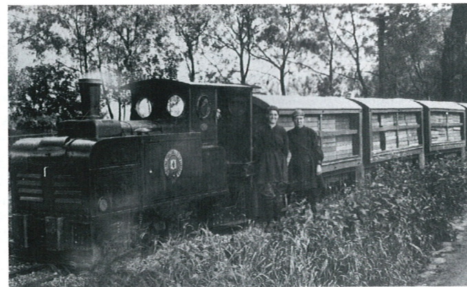
One of the Ruston, Proctor oil-fired locomotives with a train of cordite trucks in 1917.
