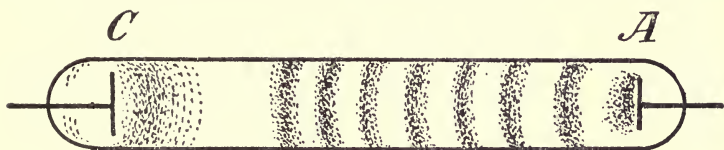
FIG. 47. ELECTRIC DISCHARGE UNDER REDUCED PRESSURE. C = Cathode. A = Anode.
