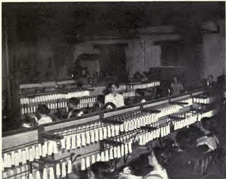
FIG. 73.—VOLKER LIGHTING CORPORATION, LTD. SEASONING UPRIGHT MANTLES.
