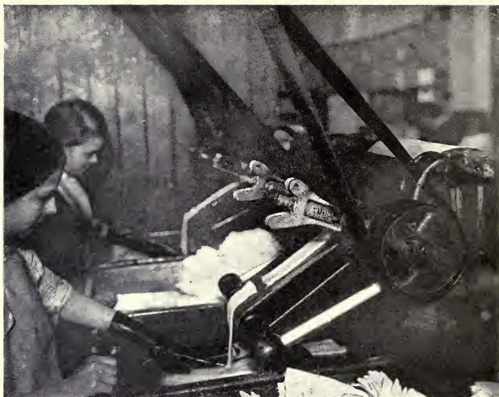
FIG. 71.—VOLKER LIGHTING CORPORATION, LTD. IMPREGNATING MANTLES
