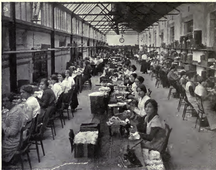
FIG. 75.—VOLKER LIGHTING CORPORATION, LTD. SEWING INVERTED MANTLES.
