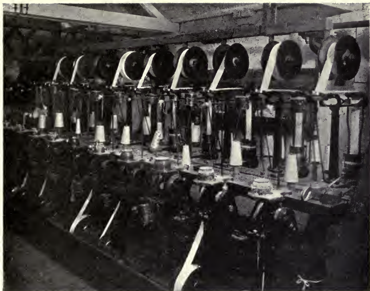
FIG. 69.—VOLKER LIGHTING CORPORATION, LTD. KNITTING THE HOSE.
