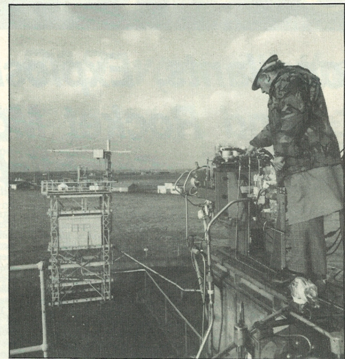
Above: preparing a rocket motor for measurement of exhaust plume structure on the special test firing tower at Westcott
