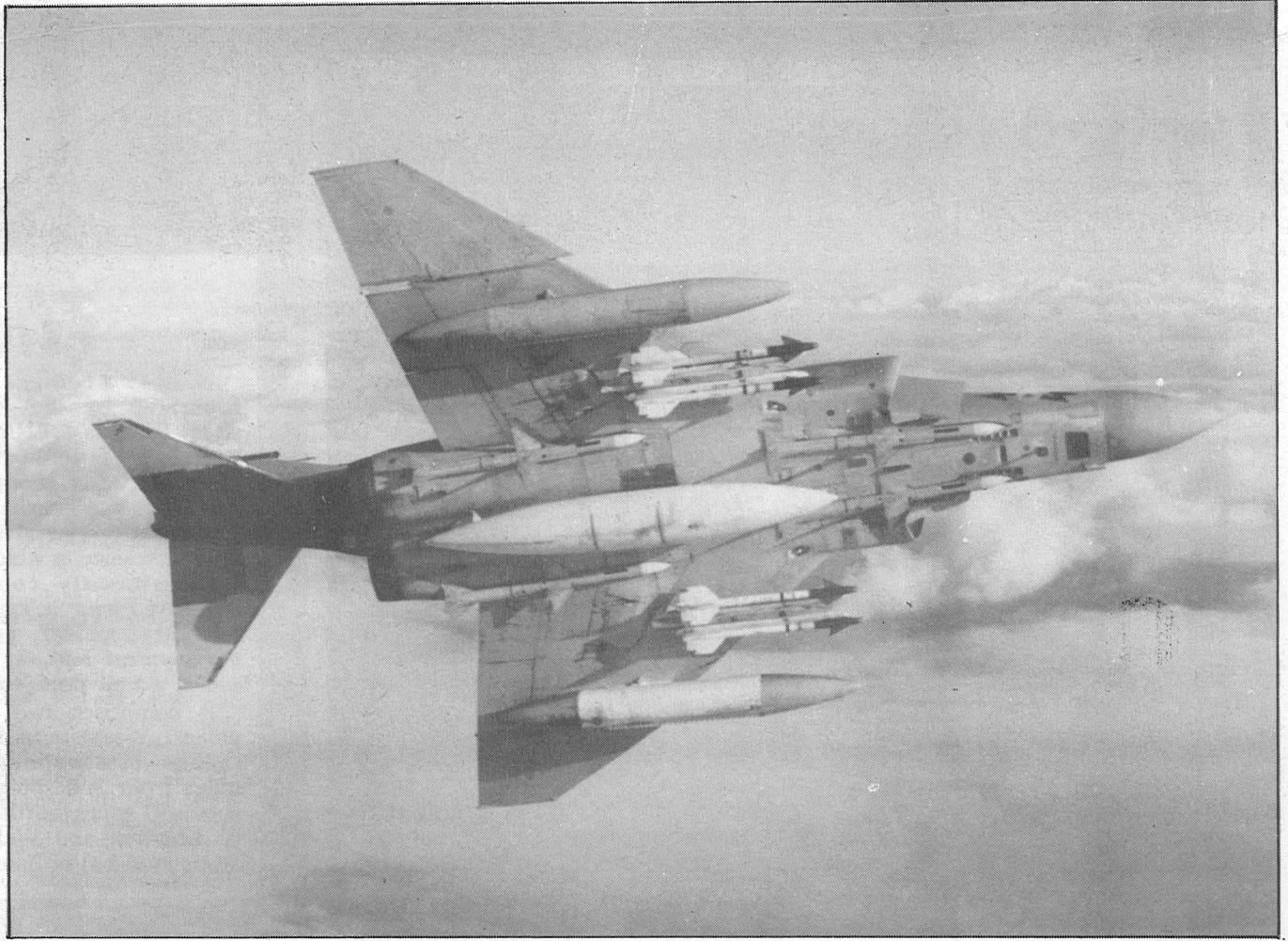
This dramatic view of an F-4 Phantom of 111 Squadron clearly shows the armament of four Skyflash and four Sidewinder missiles as well as its three external fuel tanks for increased range. The aircraft is painted in the new all over light grey low visibility camouflage with pink and light blue roundels
