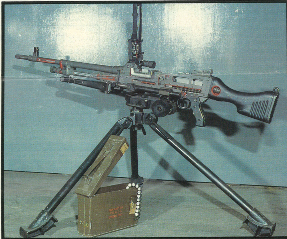
Above: Familiar environment for the GPMG as two soldiers prepare to fire it in a field demonstration. Below: This "skeleton" GPMG has key sections of body, barrel and gas tube cut away to show clearly the internal components
