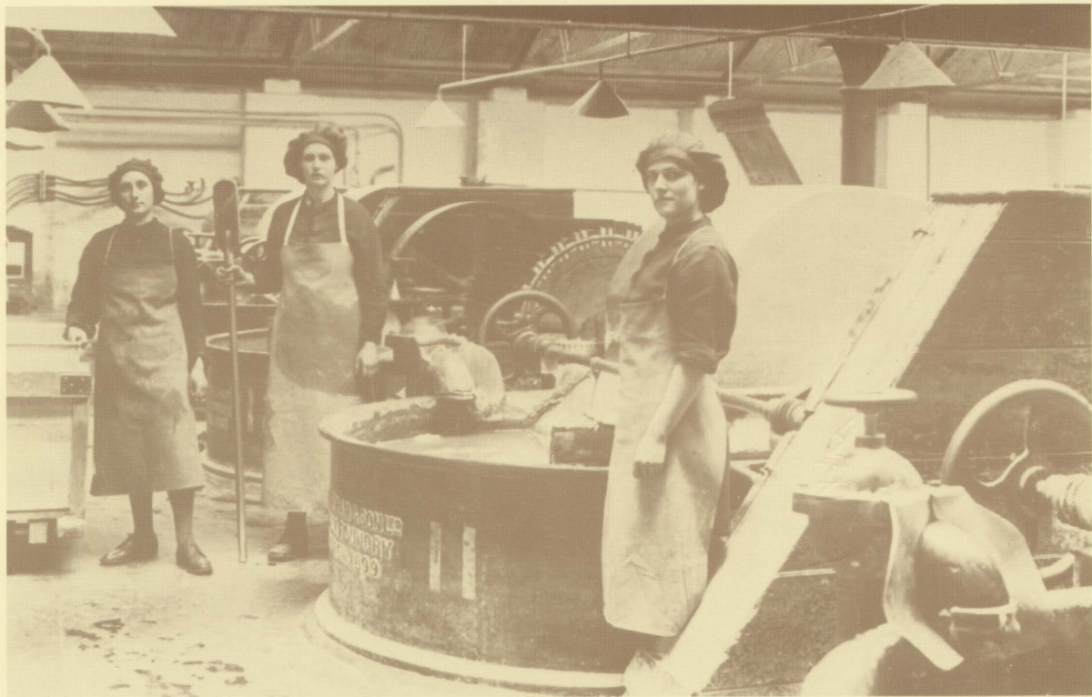
Women workers operating the guncotton pulping plant. Royal Gunpowder Factory, Waltham Abbey, 1917.
