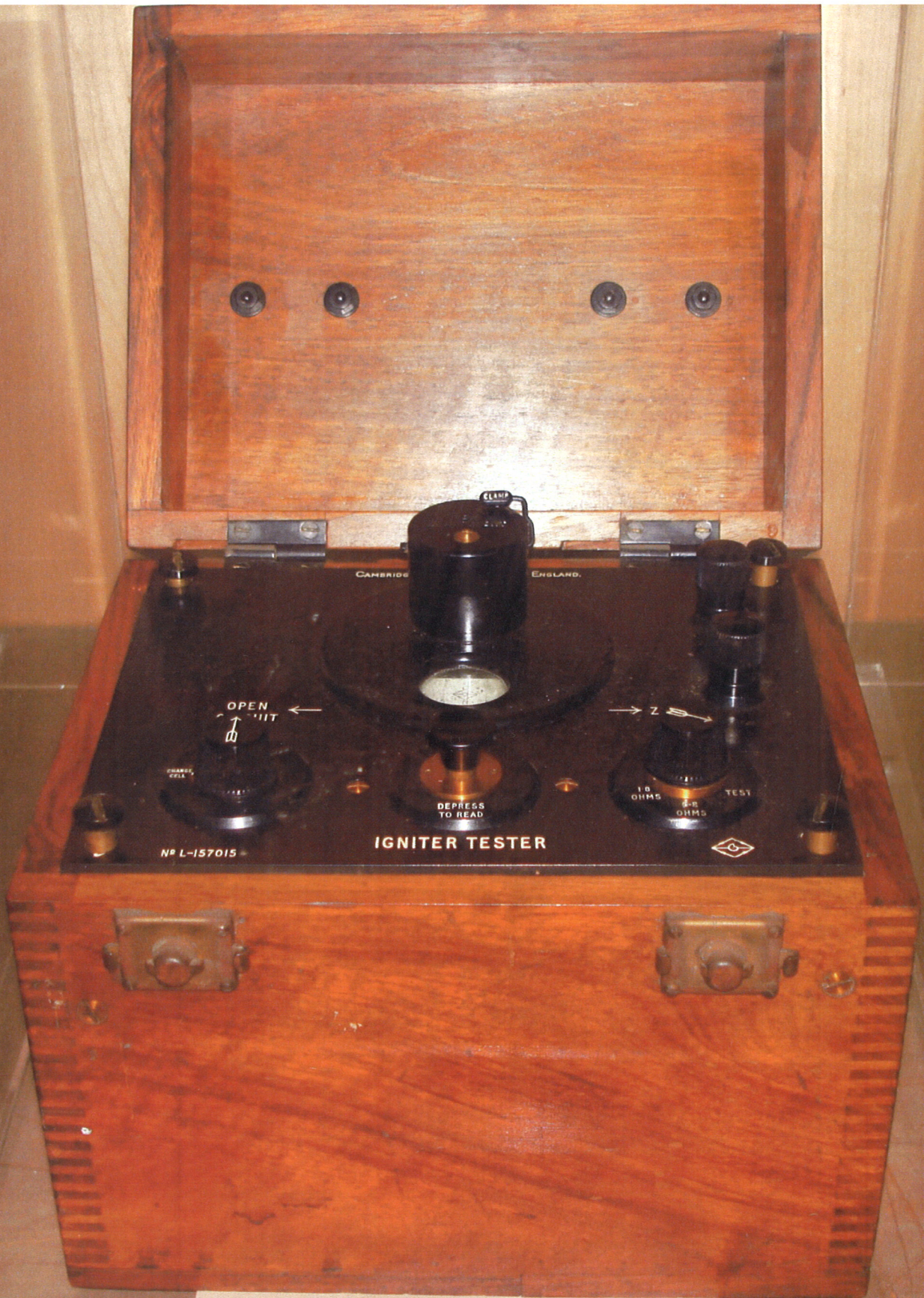
Igniter tester made by the Cambridge Instrument Co Ltd WASC 1651
