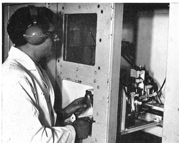
Manipulating small 10 gram mixer for sensitive high explosives. (Part of the safety screen is opened for the purpose of photographing the equipment.)
