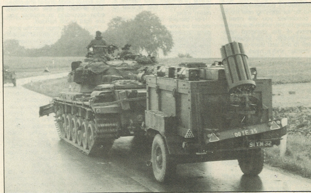
Activity is intensifying as preparations hot up for the planned counter-attack. An armoured formation has encountered an enemy minefield and Giant Viper is being towed to the location to blast a safe passage through
