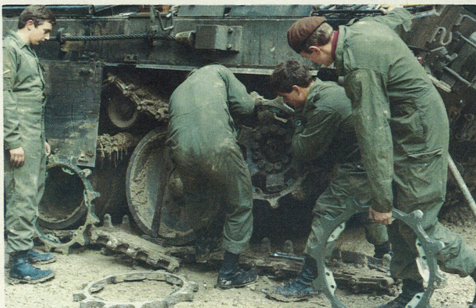
Left: As well as practising all aspects of mobilisation and combat, an exercise also tests technical support roles, such as servicing and repair of equipment. These soldiers are proving their efficiency in changing a sprocket in the field
