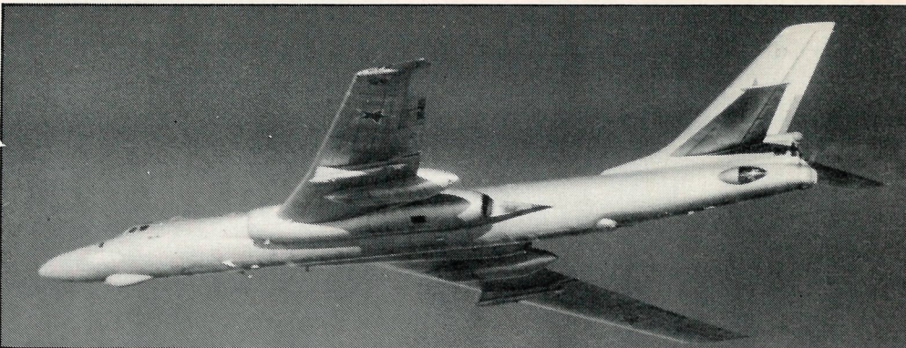
Above: Another shot of a "Bear-D" taken during a QRA interception. Below: A Soviet "Badger-C/D" — the Tupolev Tu-16 which began service life in 1955 as a strategic bomber. In various marks it has served as a missile platform, air refuelling tanker and of course a surveillance and electronic intelligence gathering (Elint) aircraft
