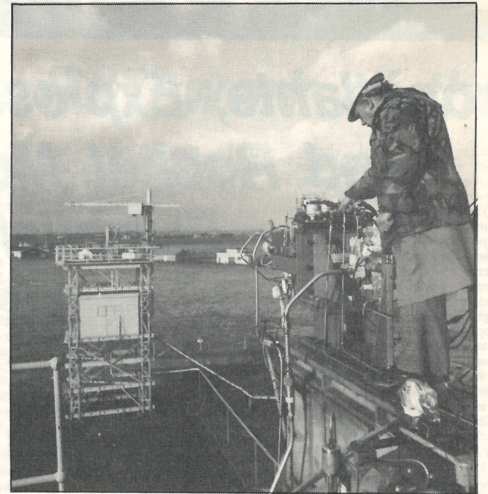
Above: preparing a rocket motor for measurement of exhaust plume structure on the special test firing tower at Westcott
