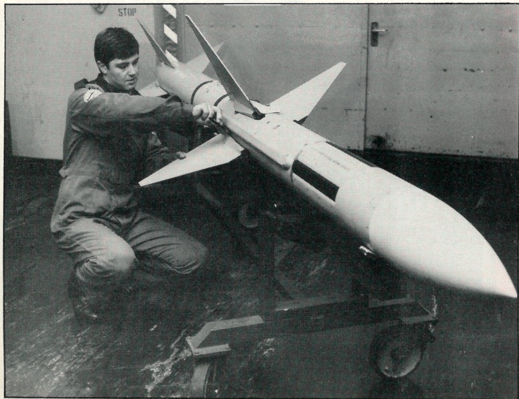
To avoid damage missiles are stored without their fins attached. This Skyflash is now required for installation on a Phantom therefore a weapons technician is securing the forward fins as part of the preparations for its deployment
