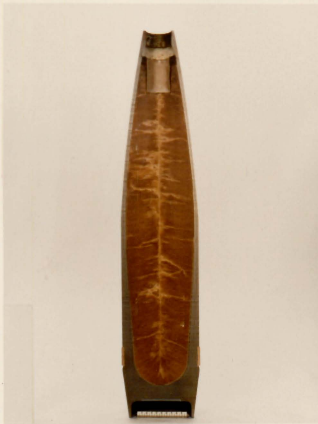
Large shell fillings of TNT based explosives can crack during manufacture.
