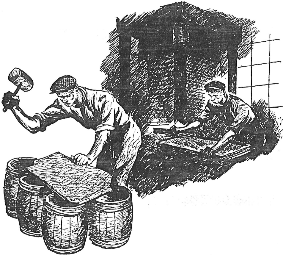
Blackpowder is chiefly needed in the form of grains. For this the powder at Roslin was first pressed into cakes, which were broken up by hand with a wooden mallet and then further reduced in size by a "corning" machine.
