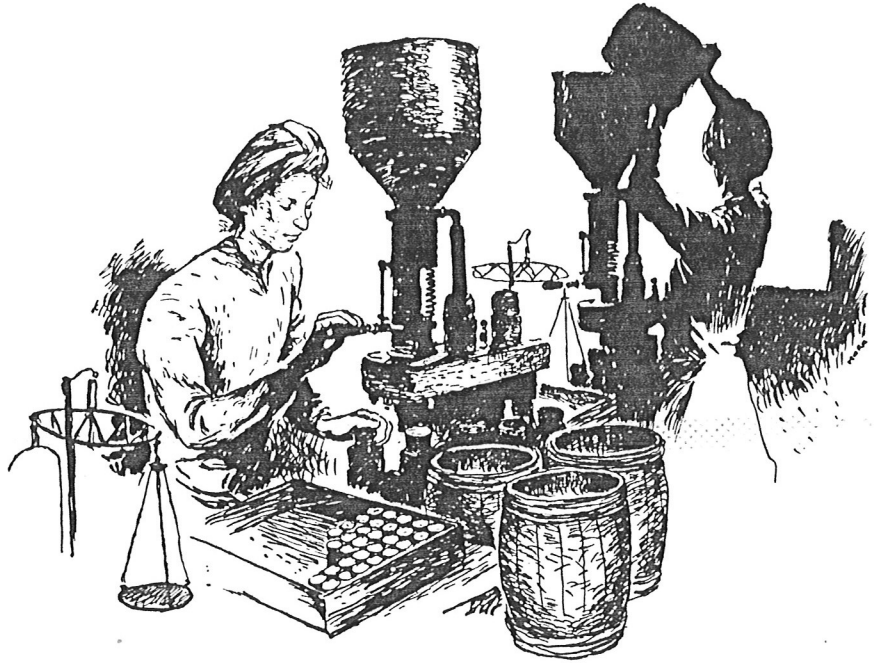
Blackpowder is here being pressed into pellets. The demand for blackpowder in pellet form comes chiefly from shale mines.
