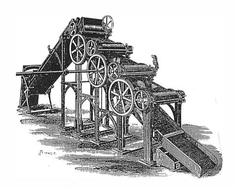
8. Corning or granulating machine with four rotating pairs of cutting rollers which are 7 ins in diameter. These have rectangular screens below them to carry the gunpowder from one pair to the next. Constructed by Taylor & Challen of Birmingham; from *Engineering* of 1878.
