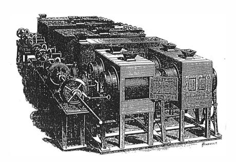
9. Set of four glazing barrels, in the foreground, each of which holds 400 lbs of powder, glazing taking 5 to 6 hours. There are reels for removing dust from large grained opowder, in the background. Constructed by Taylor & Challen of Birmingham: from *Engineering* of 1878.
