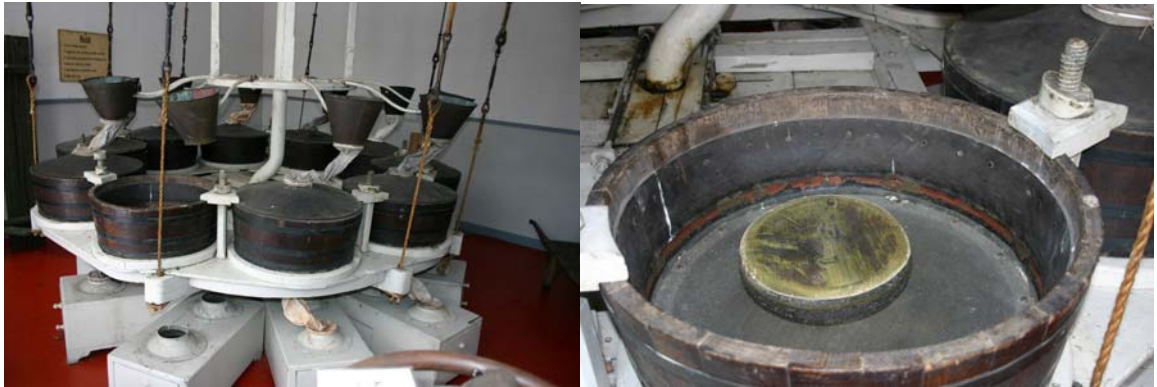
Lefebvre graining machine with 10 copper funnels and sleeves leading the powder plates down to the barrels with bronze sieves and a beech disc on each sieve pressing the grains down into the boxes beneath. To the right is a close-up view of one of the sieves.
