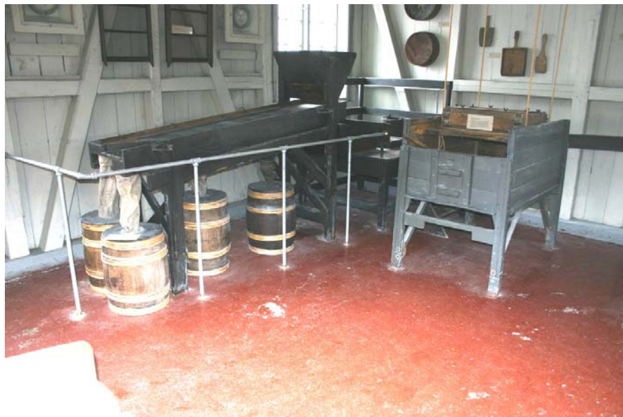
The smallest of our sorting machines in the background and a hand operated corning machine to the right. The sieves on the wall were originally woven from silk but now are of nylon.
